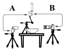
In Flash Mode, MIOPS Splash can trigger both the camera and the flash if you make the cable connections A and B.
