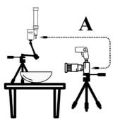
In the Camera mode, MIOPS Splash will trigger your camera only. You need to connect the camera connection cable from MIOPS Splash to the shutter release port of your camera.
