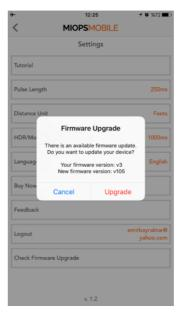
If you want to upgrade the firmware, touch the "Upgrade" button. At this point, the MIOPS Splash must be in "Firmware Upgrade" mode. In order to put MIOPS Splash into "Firmware Upgrade" mode, do the following:
