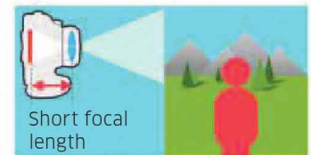
Subject takes up less of the frame using a short focal length.
