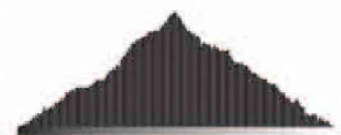
Low contrast One narrow peak indicates that the scene is very low-contrast.
