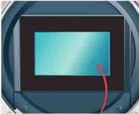
Sensor is exposed to light when the shutter is open
